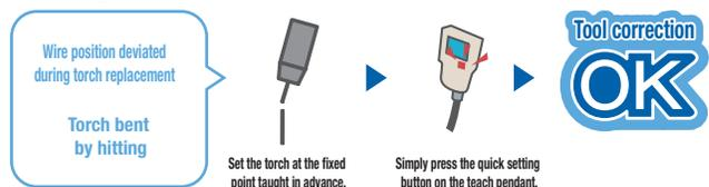
This process eliminates the need for adjustment with torch gauge, significantly reducing robot down time.
