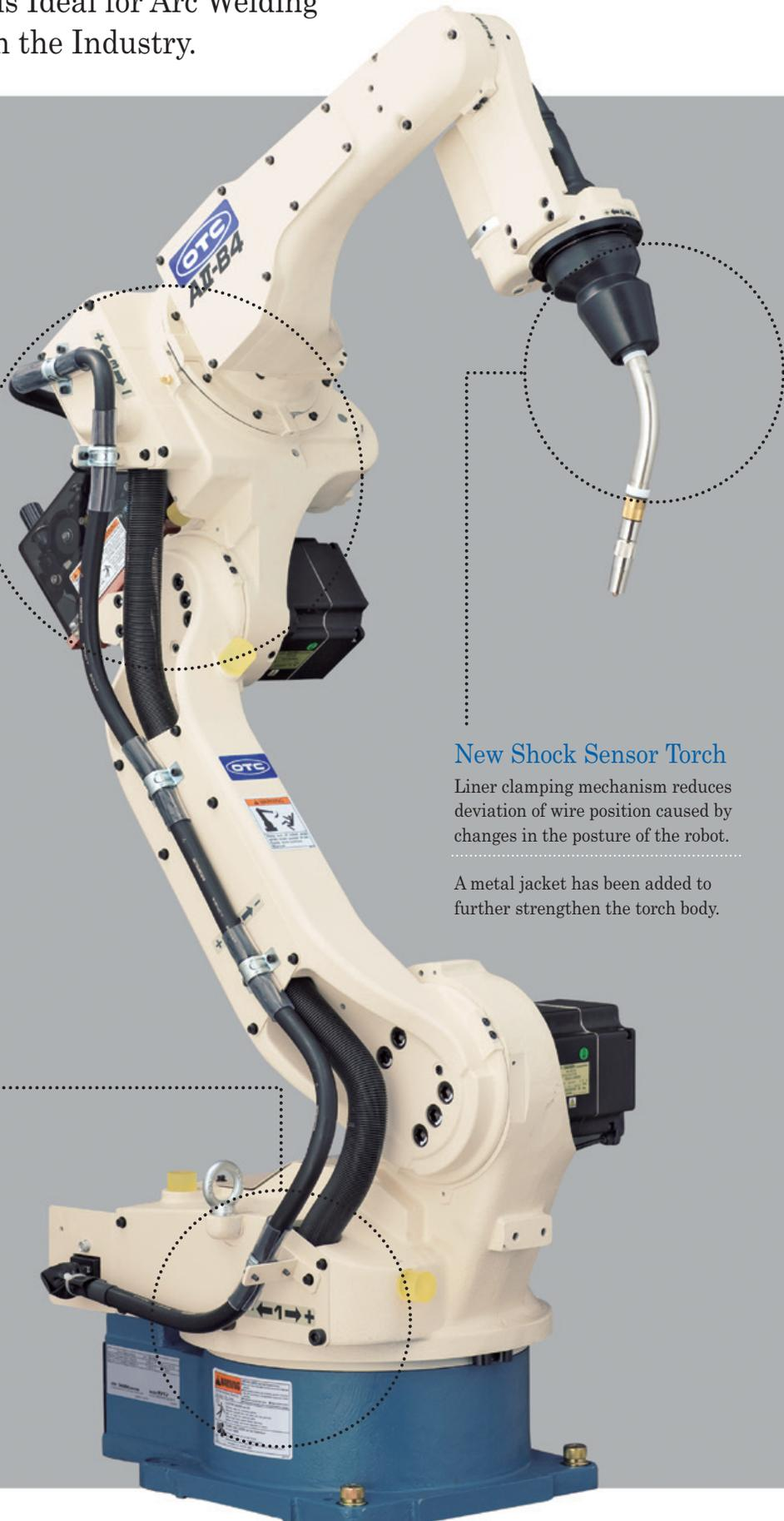
Through-arm Cable Design Provides Incredible Welding Performance, Operability and Maintainability for the Ideal Arc Welding Solution.
