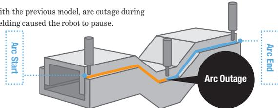
AX21 allows automatic restoration of robot operation under predefined conditions, such as the restart position and number of restarts.
